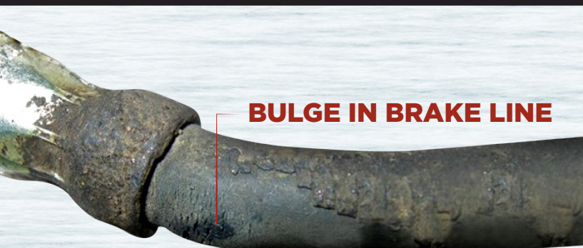
NEW MULTI-LAYER RUBBER BRAKE LINE VS DEGRADED LINE
