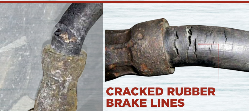
COLLAPSED RUBBER BRAKE LINE
